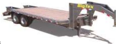
Typical gooseneck w/ loading ramps
